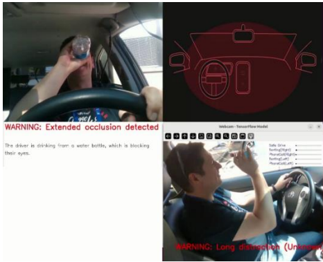
Fig. 6. Visualization of the occlusion-aware DMS. A prolonged face occlusion (3+ seconds) caused by the driver drinking water stops gaze prediction (upper right). The VLM diagnoses the cause (lower left) while the distraction detection module simultaneously warns of a "long distraction" (lower right).
