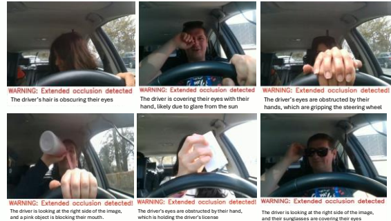
Fig. 7. Examples of occlusion detection and understanding. From left to right and up to down: Hair covering the face, hand scratching eye, hands on 12 o'clock position, drinking, holding a card and dark sunglasses.
